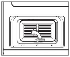
■ Turn the lever on the condenser unit upwards to the vertical position.
